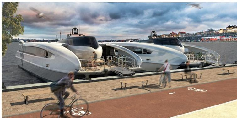
Green City Ferries (“**GCF**”) has launched the BELUGA 24, a revolutionary zero emission passenger ferry which is set to service the Swedish city from 2023. The aerodynamic, twin-hulled catamaran will have a capacity of 150 passengers and 30 bicycles.
