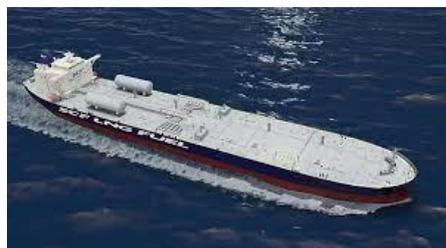
China State Shipbuilding Corporation Limited's (CSSC) first liquefied natural gas dual fuelled very large crude carrier for COSCO Shipping began sea trials recently. The vessel is 332.6 metres long and has a deadweight tonnage of 318,000. The vessel is a dual fuelled VLCC and uses LNG as its main fuel which is further supplemented by fuel oil. The vessel is also equipped with dual-fuel generators and dual-fuel boilers.
